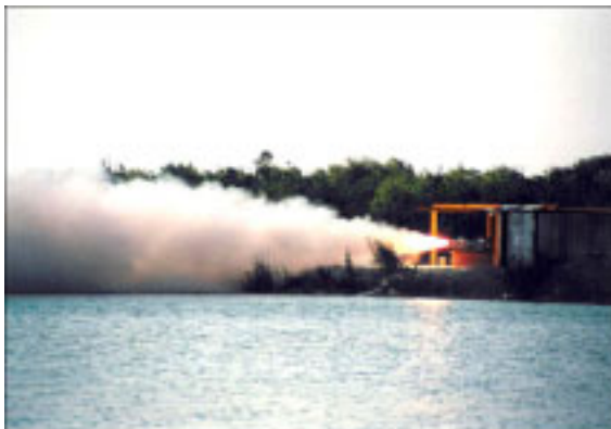
Figure 4b. Engine Firing Test (8000 lbf class)
